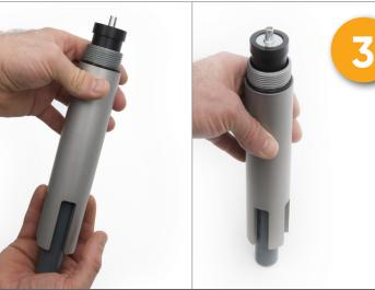
Use the plastic tube to push the old sensor head out of the sensor body. Next, apply grease to the two O-rings (one on the replacement sensor and one on the housing). You can now proceed to insert the new sensor in the housing!
