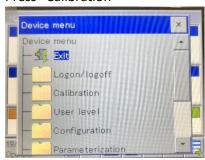
Select the sensor you want to calibrate, then press "Zero-point calibration"
