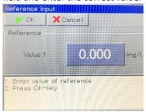
Press "OK" to accept the new zero calibration value
